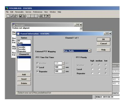
Make sure to click "ok" then write the station. None of the settings are stored until they are written back to the station. Upon completion of the write operation, the station will reset. Of course, other
