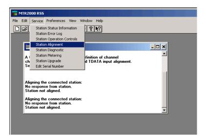
It will take a few seconds as the RSS reads alignment information from the station. To adjust RX audio, select the "Discriminator" button under "Audio Input/Output".
