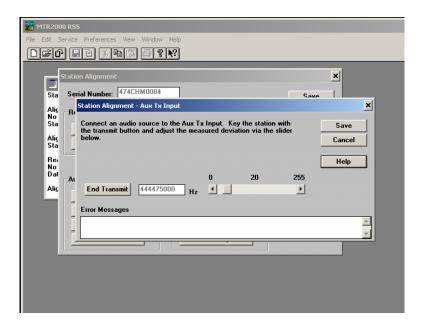
Note: When adjusting Aux TX Input, the slider will not appear until you click the "Transmit" button. The slider appears when the station is keyed. The final result will be around 26, making that a good place to start.
