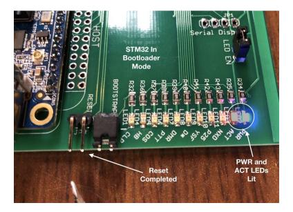
Once the board has successfully been reset and is in bootstrap mode, the **power and activity LEDs will remain lit on the STM32F446**, while only **the power LED will be illuminated on the STM32F405**. The **DMR and COR LEDs are dimly lit on both boards**; it may not be possible to see them lit in a well lighted room.
