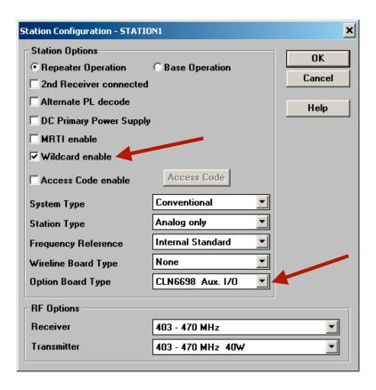
The MTR2000 SCM communicates with station modules (including the CLN6698 Auxiliary I/O board) via a Serial Peripheral Interface (SPI) synchronous serial bus operating in SPI mode 3 with 16 bit datagrams. The original CLN6698 exposed two separate SPI "slaves" to the bus, one for the inputs and one for the outputs. In each case, two 8-bit shift registers connected in series forms the hardware interface to convert parallel I/O (GPIO lines) to serial data on the SPI bus.
